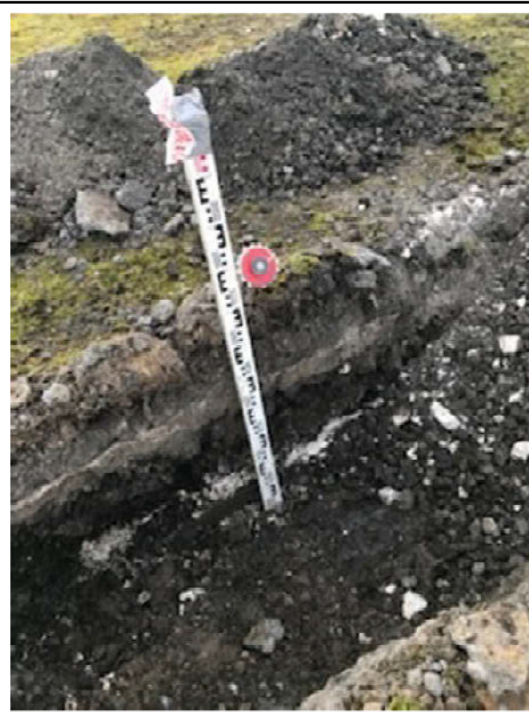
CBR at 550mm (Sub grade clay fill) 11%
