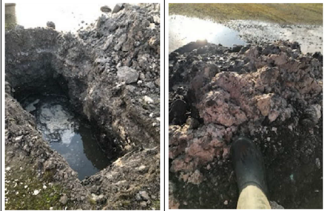
TP06 (Stone over geotextile) CBR at Ground Level after cleaning off organic layer >100%
