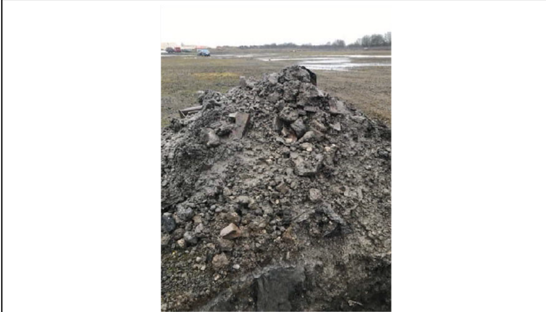
TP10 (stone over geotextile, fill is demolition and excavation arisings)
